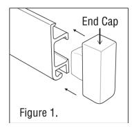
Push the End Cap into the end of the Slimline track (see Figure 1) with the curved section of the End Cap at the bottom.
