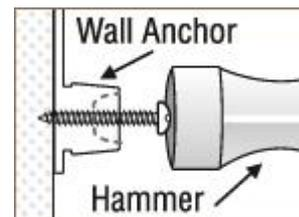
If there is no stud, drill the hole out to 6mm (1/4") and fit a "Wallmate" fitting. Then fix the wall anchor using a 25 x 8-gauge screw.
