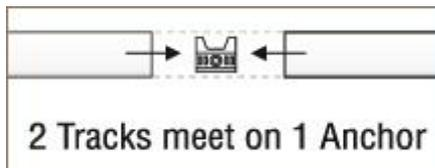
When installing two or more lengths of track continuously along a wall we suggest you use just one wall anchor to support both track ends where they join. This will ensure the two ends are perfectly aligned.
