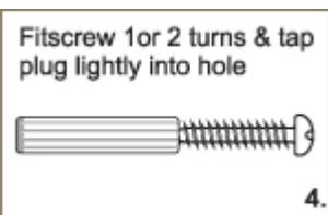
It is often hard to drill holes into masonry accurately as the drill tends to move off target. Consequently, we suggest the following:
