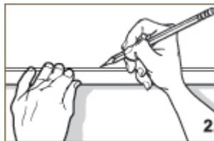
Decide on the height at which you would like the track. **IMPORTANT:** If you plan to install our lighting system leave at least 15mm between the top of the track and ceiling to allow space to fit the light wand.
