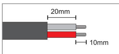
Trim the ends as shown being careful not to cut into the copper wire. Twist the bared ends of the wires and fit into the two available holes in the connector inside the Junction Box and tighten the screws. Put the lid in place so the blue cables fit into the side slits and screw the lid down.
