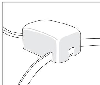
First peel the paper cover from the Double-sided Adhesive Tape you have already fitted into the track. On smooth surfaces the Junction Box can be fixed in place using the adhesive tape fitted to the back. On rougher surfaces screw in position. Fit box into the 58mm gap you have left in the track so the blue cable is level with the double-sided tape in the track. Now lay the blue cable into the track taking care it lies straight and press down firmly.
