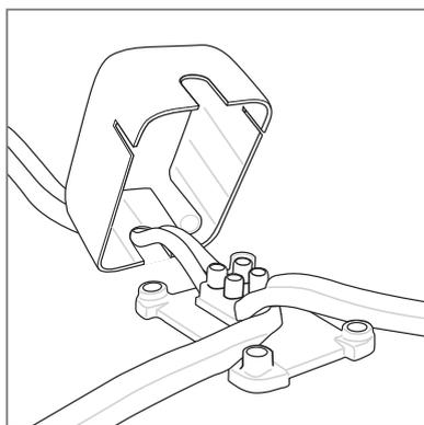
If transformer is fitted BELOW THE TRACK Measure cable length to the outside of Junction Box and add 50mm extra. Strip insulation as shown below.
