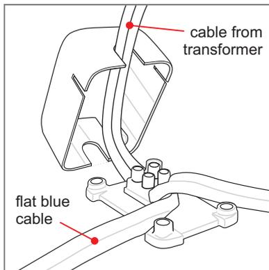
If transformer is fitted ABOVE THE TRACK Measure cable length to the outside of Junction Box and add 30mm extra. Strip insulation as shown below.
